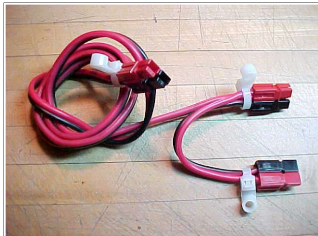
As shown here, an additional set of connectors on one end allows endless number of devices to be connected (of course keeping in mind the amount of current being drawn). I put two sets on all of my equipment. (Ed.)
