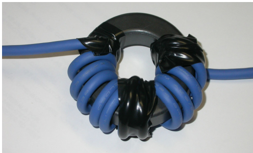
Fig 4 – A toroidal ferrite choke
