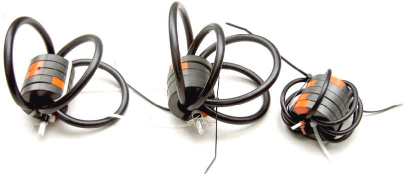
Fig 37 – Coaxial Chokes Wound to Minimize Capacitance and Inductance
