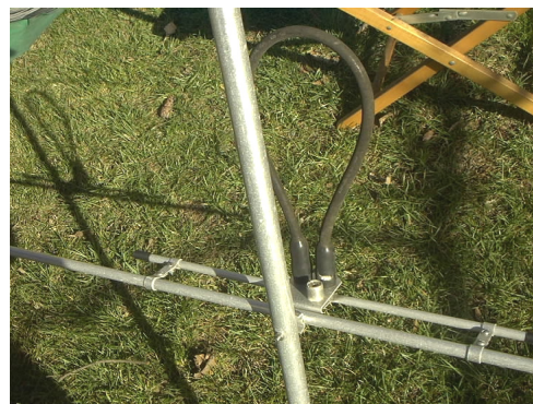
Fig 32 – A Half-Wave Balun
