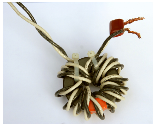
Fig 30 – A line filter for 1-14 MHz
